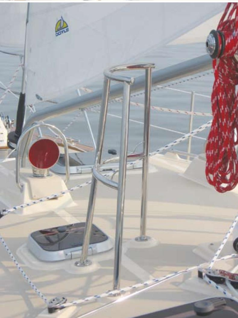
**The spacious aft deck, top, is the perfect place for relaxing at anchor or for stowing the dinghy while underway. Sturdy stainless steel stanchions, above, increase safety while at the mast**
