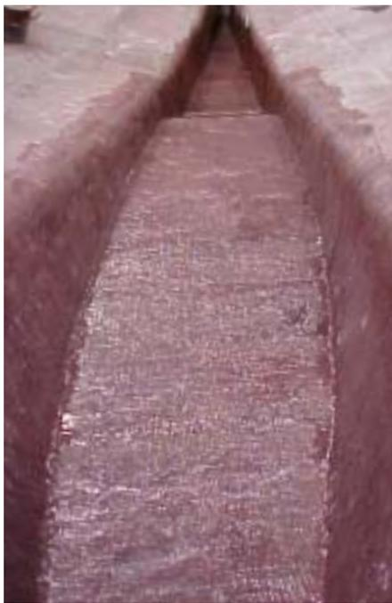
The assembly process begins with the addition of ballast to the keel. One of the advantages of an integrally molded full keel is that a significant portion of the ballast can be placed very low, along the length of the keel, much like a long, encapsulated “bulb” at its base.
