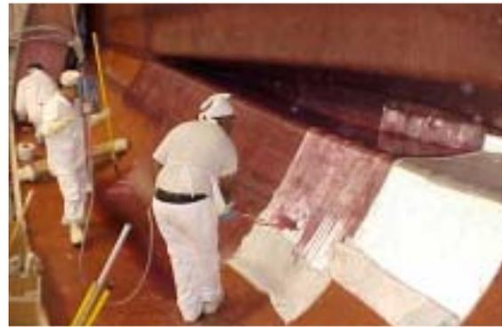
Applying the glass and resin layers by hand allows for a great deal of quality control. More importantly, it allows the use of high modulus fabrics, which provide high glass-to-resin ratios and superior impact resistance.
