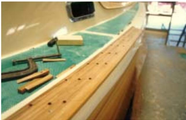
The teak toe rails, which are hand formed in our mill, are then fastened and sealed with 3M® 5200 sealant and stainless steel screws. Stanchions, cleats, rails, and genoa tracks are all mounted to the toerail and thru-bolted to aluminum backing plates.
