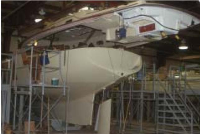
When the interior nears completion, the deck / headliner unit is moved into place for installation. The process begins with the precise fitting of the headliner to the tops of the structural bulkheads. Even though the deck and headliner are made from fixed molds, the decking crew goes through the painstaking process of custom fitting this unit by lowering it, marking the bulkheads, raising it, and trimming the bulkheads. This process is repeated until a precise fit is achieved.
