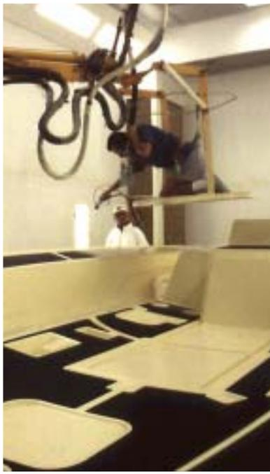
The lamination process begins in a room dedicated to gel coat application. Before the gel coat is sprayed into the mold, a releasing agent is applied to ensure a clean separation of the finished part. The molding process seems a little backwards as the gel coat -- the outer coating -- is actually applied *before* the fiberglass and resin layers.
